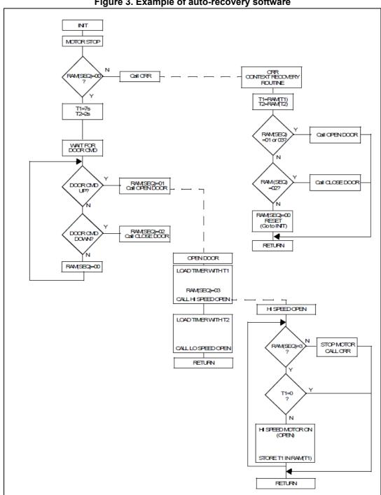
Figure 3. Example of auto-recovery software
