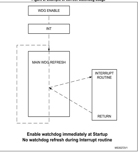
Figure 2. Example of correct watchdog usage
