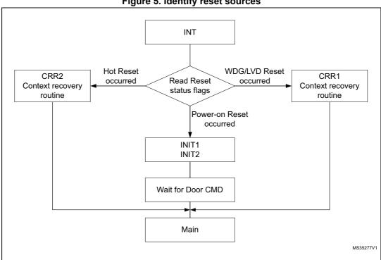
Figure 5. Identify reset sources
